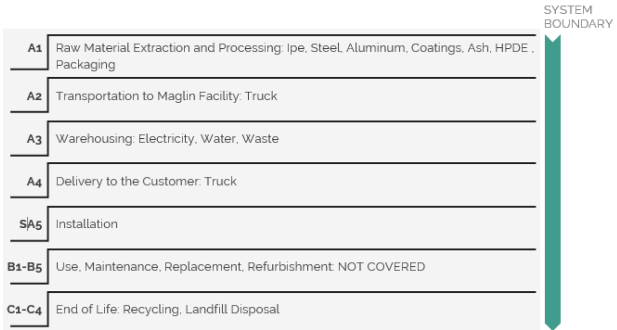
Figure 2: General system inputs considered in the product system and categorized by modules in scope
